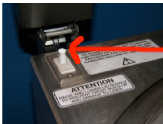
Figure 1 -- Lid Switch on the MVE Freezer Series
